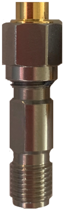
Figure 15: Photograph showing the female open used in the 85033 calibration kit. The S-parameters of these are individually measured, and the data provided on the USB stick. In addition the data as a polynomial is given on the calibration certificate.
