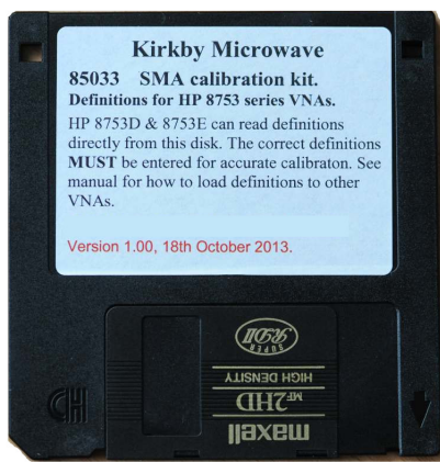
Figure 9: Photograph showing a 3.5” floppy disk that can be used to load the coefficients into some early HP or Agilent VNAs.
