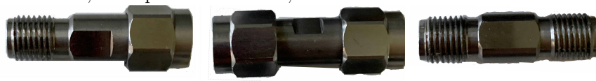
Figure 7: Photograph showing the 3 phase matched adapters. Unlike the other optional adapters for use with the 85033 calibration kit, these adapters can be used to 27 GHz, but we only phase match these to the maximum frequency of the kit ordered, which is always 18 GHz or less.
