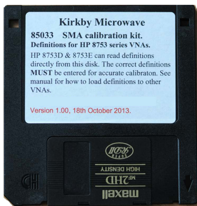
Figure 10: Photograph showing a 3.5" floppy disk that can be used to load the coefficients into some early HP or Agilent VNAs. The disk shown is is option 010 disk for the very popular 8753 series of VNAs, but all disks look similar.
