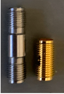
Figure 20: Photograph showing the two types of female-female thru used in the calibration kit. The delay of these is measured. These are not phase matched to the male-male thru unless option 003E is ordered, which also adds a male-female thru.
