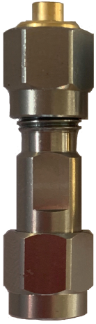
Figure 16: Photograph showing the male open used in the 85033 calibration kit. The S-parameters of these are individually measured, and the data provided on the USB stick. In addition the data as a polynomial is given on the calibration certificate.
