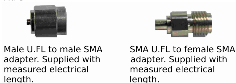
Figure 3: Photograph showing the two U.FL to SMA adapters. The upper frequency limit of the U.FL connector is 6 GHz. Normally U.FL connectors are designed for 20 matings, and mate very tightly requiring a tool to remove them. The adapters supplied use a low retention force design, which is designed for 500 matings.
