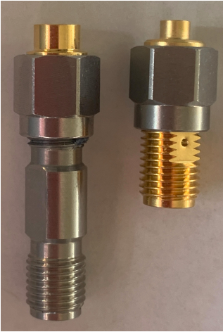
Figure 14: Photograph showing the two types of female open used in the 85033 calibration kit. The 12 and 18 GHz models use those on the left. Lower frequency kits sometimes use the female open on the right. Do not be surprised by some small differences - sometimes the open section is all gold plated.
