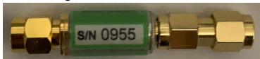
Figure 11: Photograph showing the option 023 attenuator with two male connectors. Port 1 is shown to the left, with the text up the correct way.
