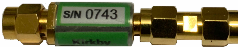
Figure 24: Photograph showing the reference attenuator with two male connectors, included in kits with option 023. The serial number will be different to that of the calibration kit.
