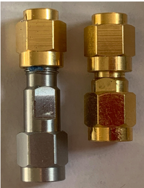
Figure 17: Photograph showing the two types of male short used in the 85033 calibration kit. The 12 and 18 GHz models use those on the left. Lower frequency kits usually (but not always) use the male short on the right.
