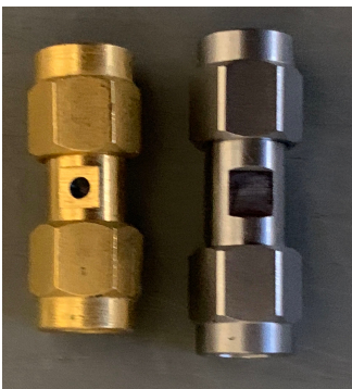
Figure 21: Photograph showing two of the types of male-male thru used in the calibration kit. The device in your kit may look slightly different. The delay of these is individually measured. These are not phase matched to the male-male thru unless option 003E is ordered, which also adds a male-female thru.
