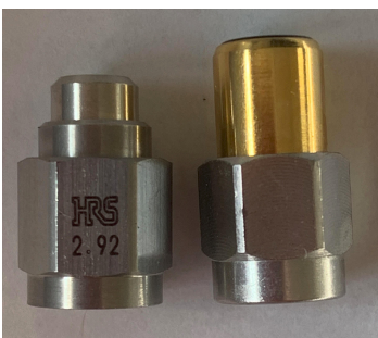
Figure 20: Photograph showing the two of several types of male load used in the 85033 calibration kit. Do not be tempted to replace the loads with a similar or identical looking device. Many loads of the same manufacturer and model number will have inferior performance. Each load is specially selected, and not all loads are suitable for calibration kits.
