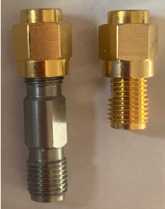
Figure 16: Photograph showing the two types of female short used in the 85033 calibration kit. The 12 and 18 GHz models use those on the left. Lower frequency kits usually (but not always) use the male short on the right.
