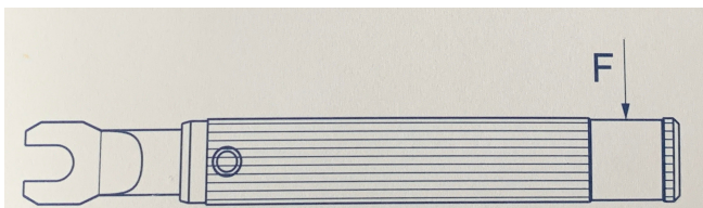
Figure 13: This shows how a torque spanner should be properly used. As one piece is tightened, the other pieces must be held so it does not rotate using a second spanner. The torque spanner and the other spanner should always be within 90° of each other.
