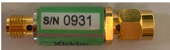
Figure 22: Photograph showing the standard reference attenuator included with every 85033 calibration kit. The serial number should match that of the calibration kit.
