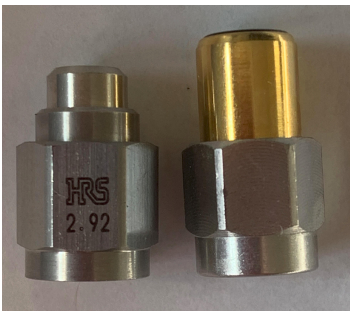
Figure 19: Photograph showing two of several types of male load used in the 85033 calibration kit. Do not be tempted to replace the loads with a similar or identical looking device. Many loads of the same manufacturer and model number will have inferior performance. Each load is specially selected, and not all loads are suitable for calibration kits.
