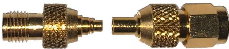
Figure 4: Photograph showing the two MMCX to SMA adapters included with kits with option 003A. The upper frequency limit of the adapters is 6 GHz. These should not be confused with the larger MCX adapters (option 003D)
