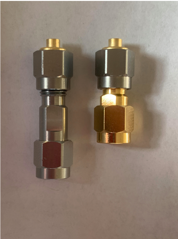
Figure 15: Photograph showing the two types of male open used in the 85033 calibration kit. The 12 and 18 GHz models use those on the left. Lower frequency kits usually (but not always) use the male open on the right.
