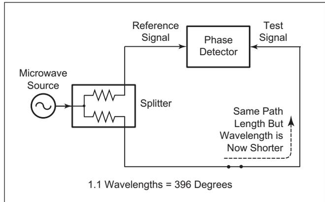
Figure 9. Split Signal where Path Length is longer than One Wavelength
