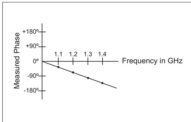
Figure 10. Electrical Delay
