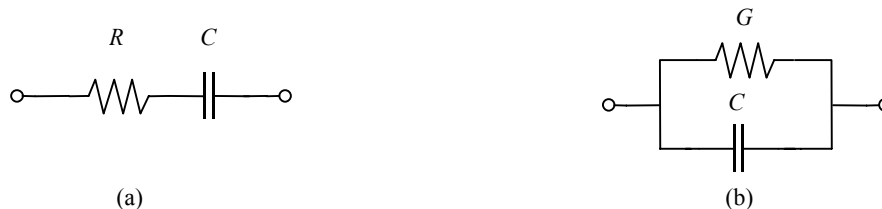
Figure 2. Simple series, (a), and parallel, (b), equivalent circuits of the dielectric specimen in the admittance cell of Figure 1. R and G take account of the dielectric loss in the specimen. R is the equivalent series resistance and G is the equivalent parallel conductance of the dielectric.
