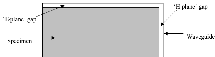
Figure 41. Air gaps around a specimen that is being measured in a waveguide cell. The Figure shows a cross-section of the waveguide with the specimen in it.
