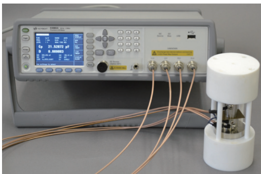
E4980A Precision LCR Meter and DPT-009 for sheet, liquid, gel
